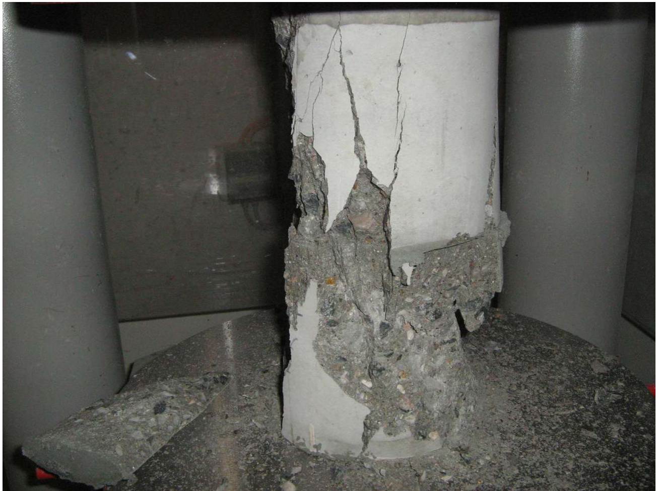
Concrete cylinder with joint after the compression test, the wedge-shaped break-out is clearly visible
